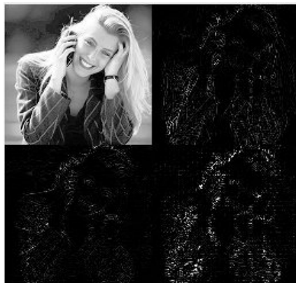
Fig. 4. 2D Lifting wavelet implementation 'phone.jpg' 256x256
