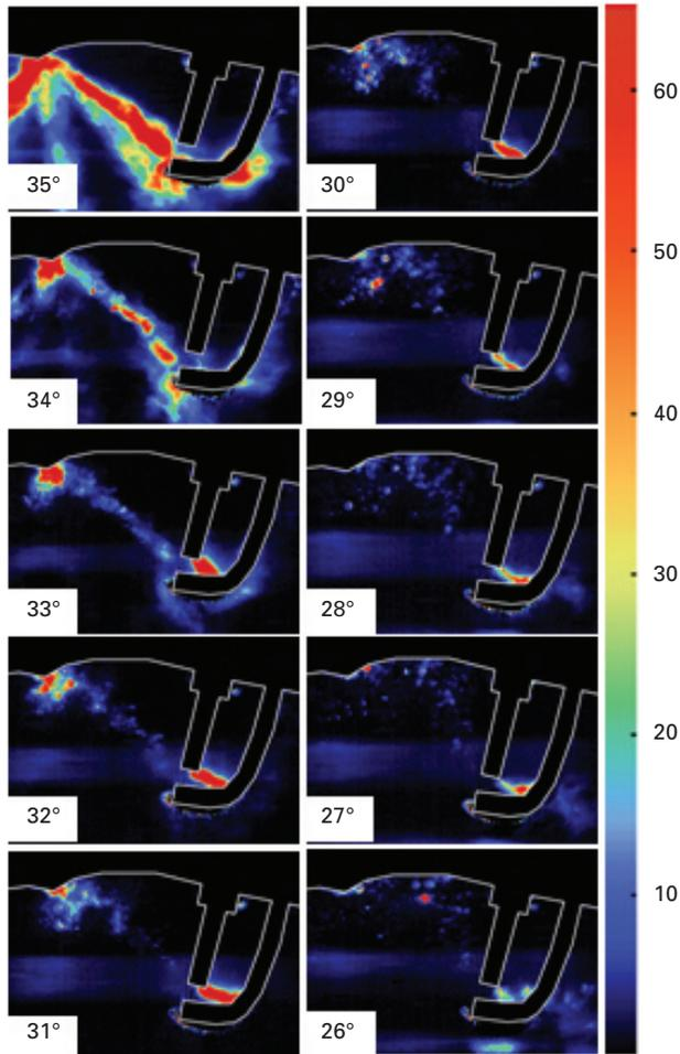
**Plate XIII** Single cycle sequence of Mie scattering images that were acquired at 12 kHz in a spray-guided direct-injection engine. The arc follows the original spray trajectory, showing the impact of the spray momentum of the development of the spark (Smith and Sick, 2006b).
