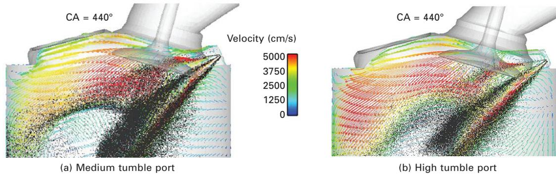
**Plate X** CFD-predicted velocity field and spray distribution for medium tumble (left) and high tumble (right) intake port designs in a turbo-charged DISI engine equipped with a multi-hole injector mounted beneath the intake ports. The operating conditions are 2000 rpm, 19 bar BMEP, split injection with 80/20 ratio between the first and second injection with start of injection of 400° and 500° aTDC, (Iyer and Yi, 2008).
