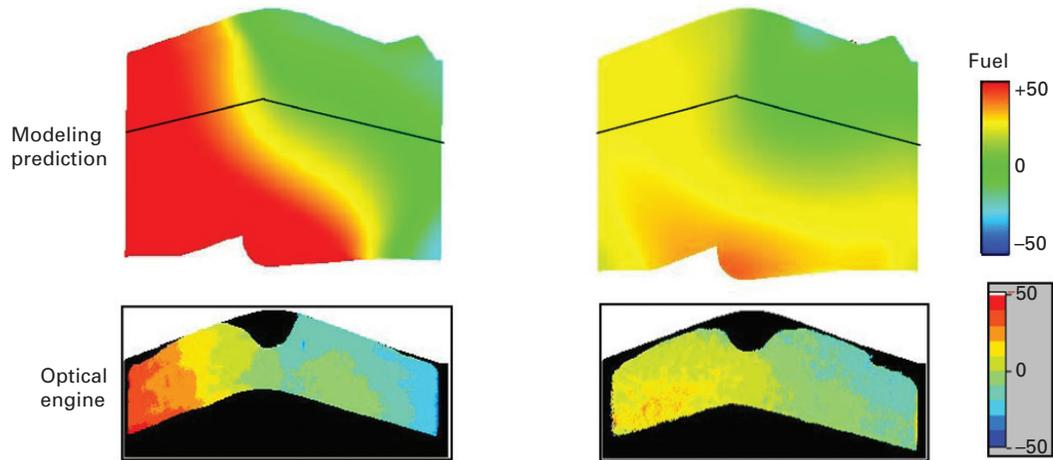
**Plate V** Correlation between modeling prediction and optical engine measurement of fuel-air mixing at  $630^\circ$  ( $90^\circ$  bTDC compression). The modeling is with constant MAP of 62 kPa. The experiment is at an operating condition of 1500 rpm, 2.62 bar BMEP. The injector has a  $60^\circ$  spray cone angle and the EOI is  $280^\circ$  bTDC (Yi *et al.*, 2004b).
