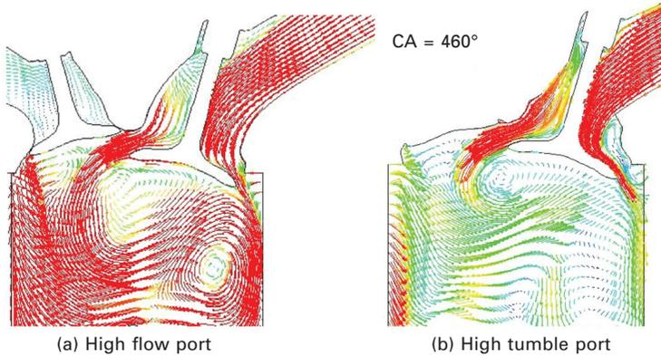
**Plate I** Comparison of near-valve flow structure between high flow port (left) and high tumble port (right). The high flow port has a more uniform velocity flow field around the valve seat area, while the high tumble port shows a more biased flow structure with flow separation on the short side of the port. The operating condition is full load at 5000 rpm (Iyer and Yi, 2008).
