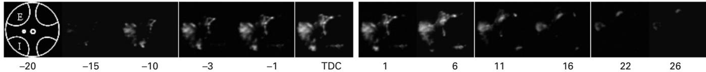
6.20 Mini combustion with simultaneous in-cylinder pressure, heat release rate and full chemiluminescence images at  $\lambda_1$ , 1600 rpm, gain 50%, SOI = 80° CA BTDC.
