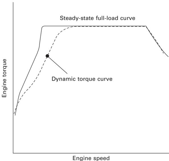
3.4 Turbocharged engine transient and steady-state torque curves.
