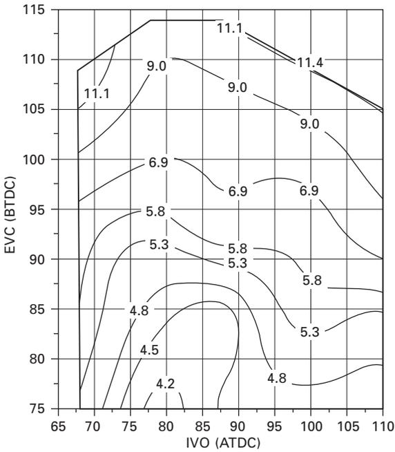
6.17 Contours of brake specific hydrocarbon emissions (g/kWh).
