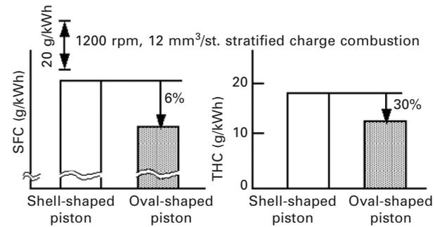
**Plate VII** CFD modeling predicted that mixture formation with an oval piston cavity is better located than in the case of a shell-shaped cavity (left), which agrees with the experimental results showing improvement in fuel economy and UHC emissions, (Abe *et al.*, 2001).
