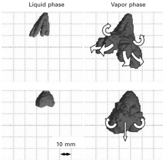
10.4 Exciplex imaging of two sprays from a multihole injector (top) and an annular orifice injector (bottom) at  $p_{\text{amb}} = 0.94$  MPa and  $T_{\text{amb}} = 220^\circ\text{C}$ ,  $t = 800 \mu\text{s}$  after start of injection (Rogler *et al.*, 2007). Reprinted with permission from SAE Paper 2007-01-1827, © 2007 Society of Automotive Engineers of Japan, Inc. and © 2007 SAE International.
