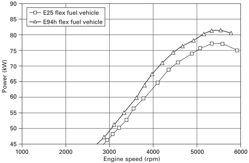
9.3 Power comparison between alcohol (E94h) and gasoline (E25), 1.6 liter engine, 4 cylinder, spark-ignited, compression ratio = 12.3:1, adapted from [35].
