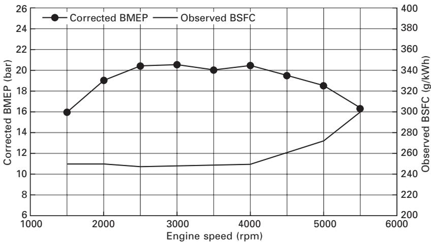
3.18 Full-load BMEP and BSFC for ‘Sabre’ turbocharged DISI engine fitted with an exhaust manifold integrated into the cylinder head (IEM). Data reproduced from Coltman *et al.* [16].
