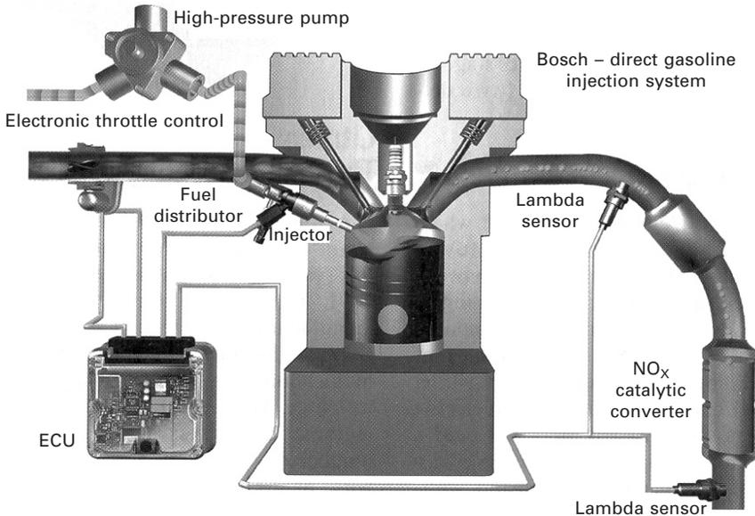
1.2 A typical DI gasoline engine.
