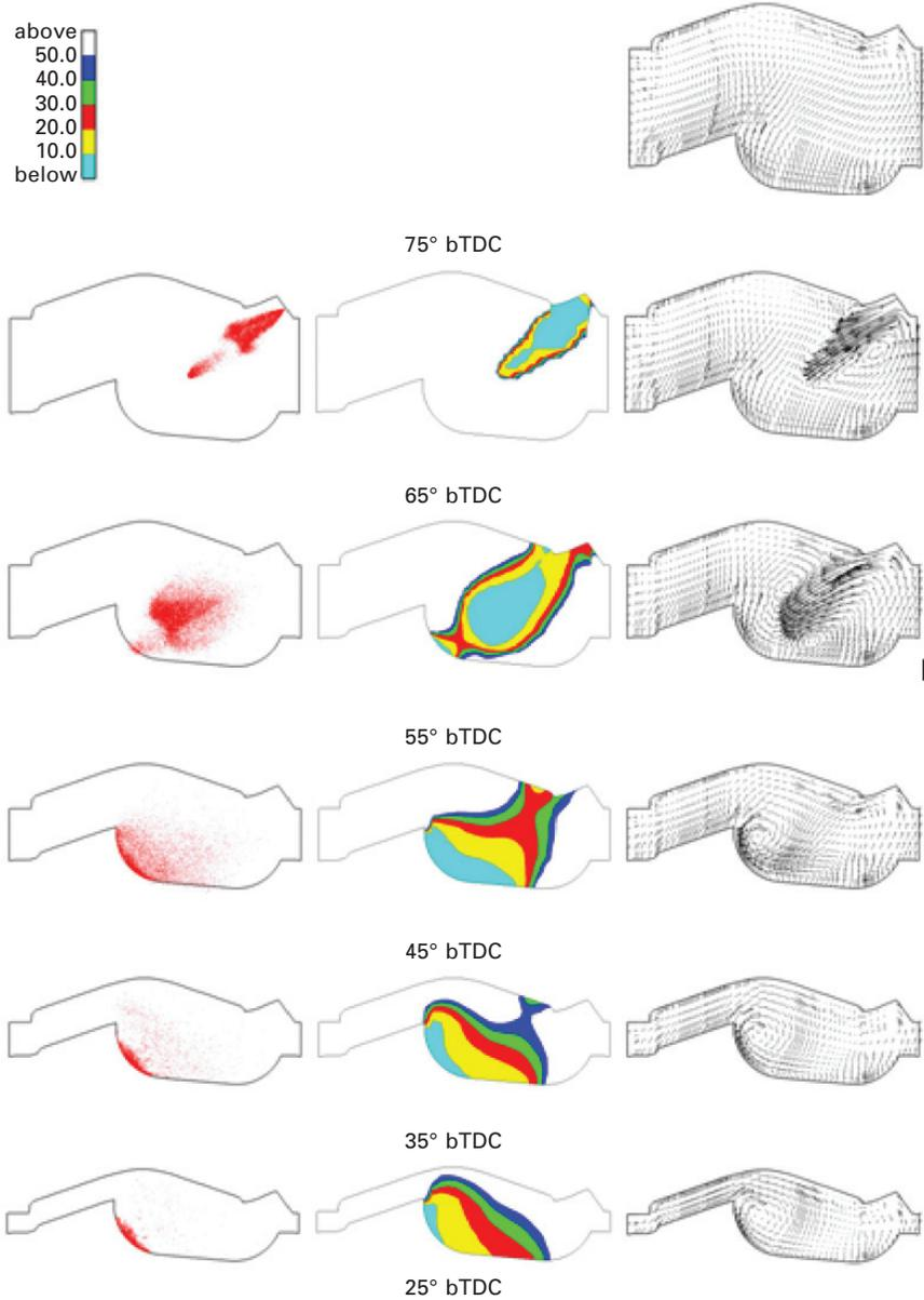
**Plate VIII** CFD-predicted evolution of the fuel spray, air–fuel ratio distribution, and gas vector field in the central plane of the combustion chamber. The simulated engine conditions are 1500 rpm, 10 mg injected fuel mass and 1.0 bar intake manifold pressure. The nominal spray cone angle is 60°, the start of injection (SOI) is 70° bTDC, the injection duration is about 8.7 crank angle degrees, and the injection pressure is 100 bar. (Han *et al.*, 2002).
