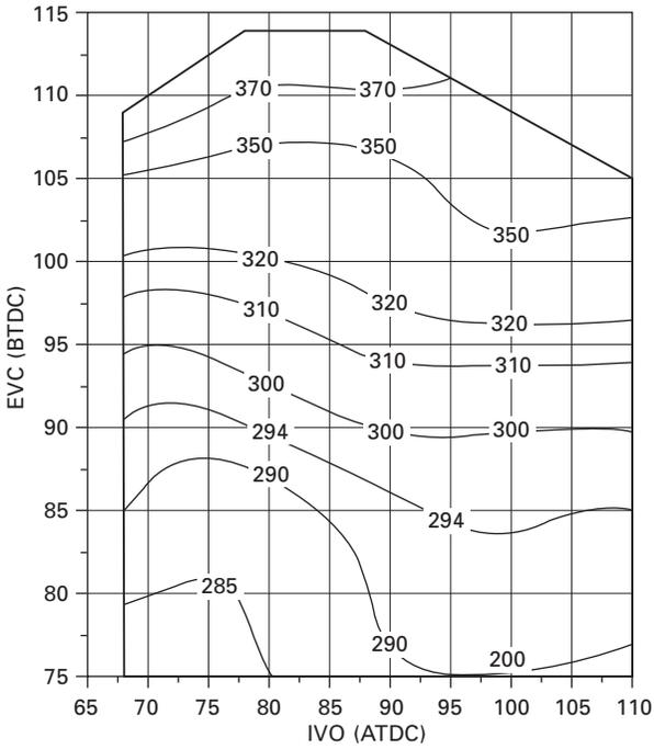
6.16 Contours of brake specific fuel consumption (g/kWh).
