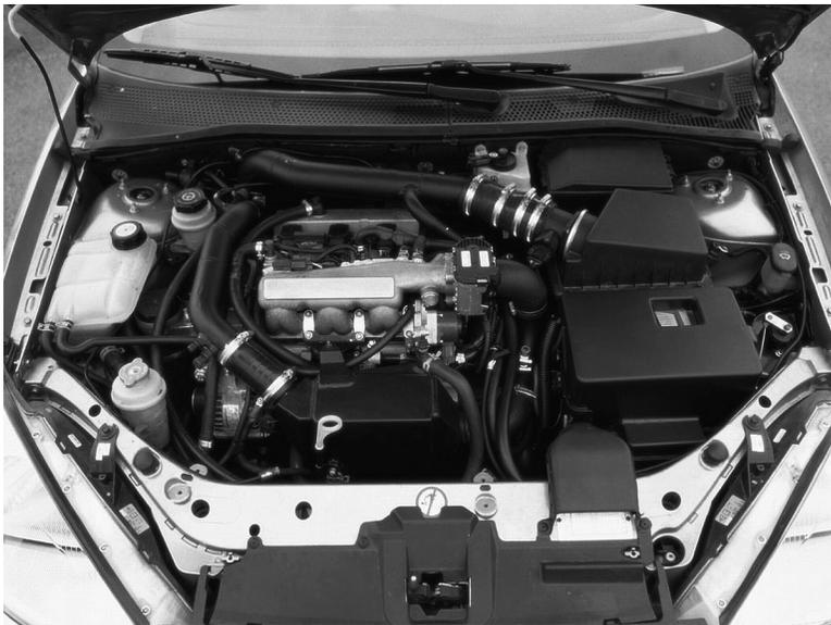
4.7 Vehicle installation of LBDI engine.
