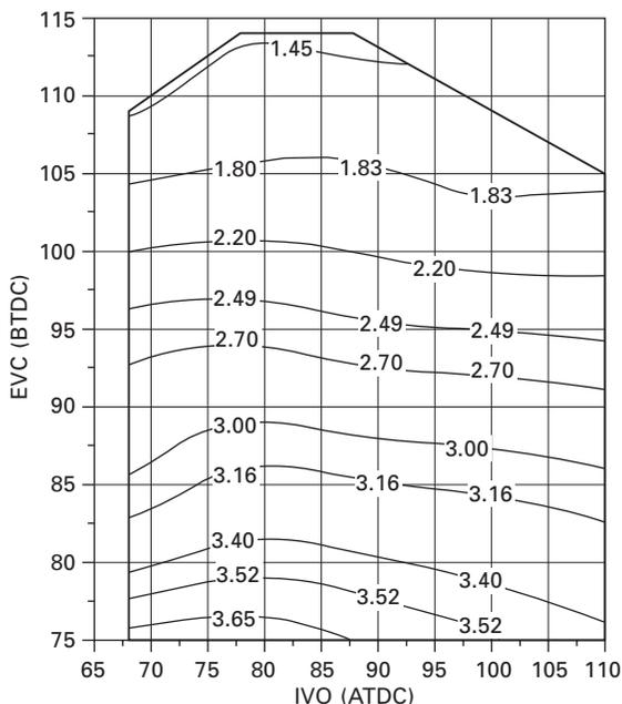
6.13 Contours of brake mean effective pressure (bar).
