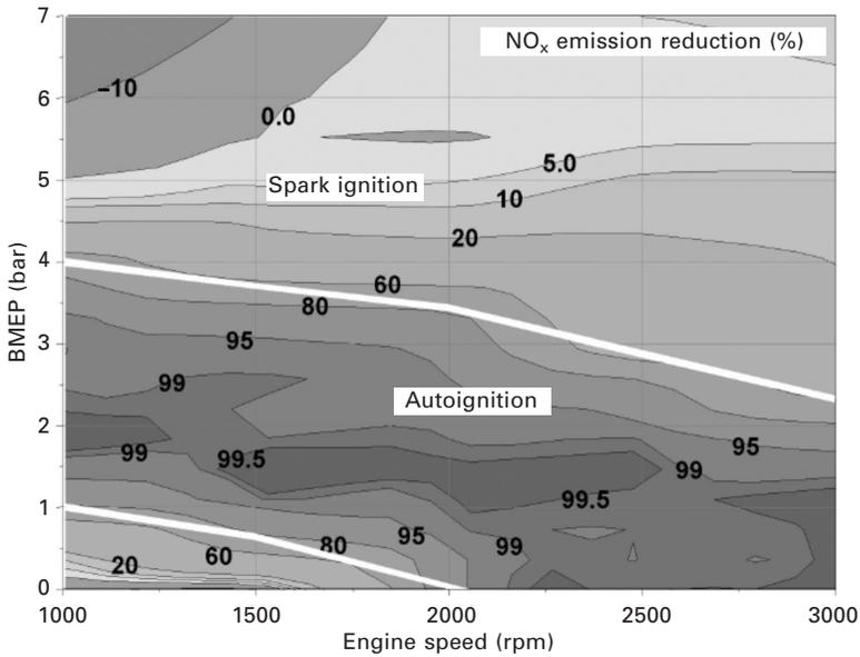
6.7 NO<sub>x</sub> emission reduction achieved with the AVL-CSI engine (adapted from Fuerhapter *et al.*, 2007).
