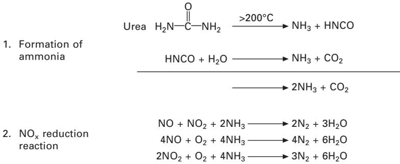
1.9 Schematic of the urea-based SCR NO<sub>x</sub> aftertreatment.
