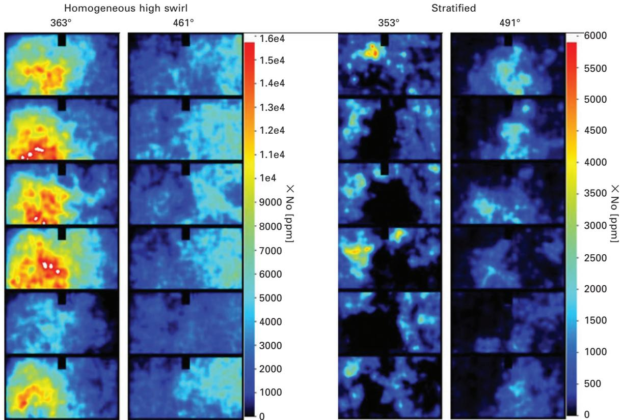
**Plate XIV** The instantaneous concentration distribution of nitric oxide in a direct-injection engine shows the strong impact of mixture preparation on nitric oxide formation. Measurements were performed with laser-induced fluorescence. (Fissenwert *et al.*, 2005). Reprinted with permission from SAE Paper 2005-01-2089, © 2005 SAE International.
