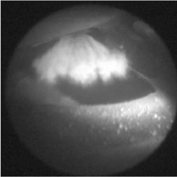
7.9 Endoscopy image taken at 26.4 CAD BTDC in an optically accessible engine, operating condition 2000 rpm,  $IMEP_n = 2.7$  bar,  $EOI_{1/2} = 29.5/23.5$  CAD BTDC,  $TI_{1/2} = 197/141$   $\mu$ s (Baecker *et al.*, 2007).
