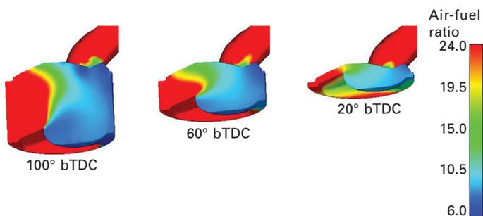
**Plate II** Air-fuel ratio distribution at 6000 rpm full load in the initial combustion system design. The start of injection is 10° After Top Dead Center (aTDC) in the intake stroke. The injection duration is about 188° and the average air-fuel ratio is about 13:1. (Yi *et al.*, 2002).
