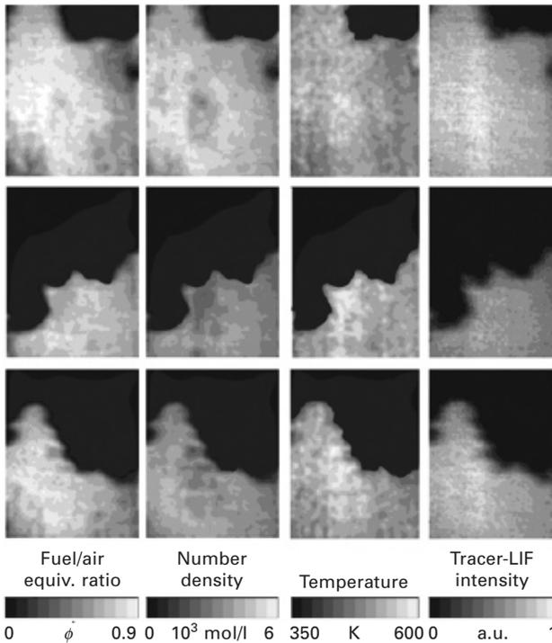
10.6 Temperature and fuel measurements based on 3-pentanone LIF imaging in an engine. Excitation at 248 and 308 nm was used for these measurements (Einecke *et al.*, 2000). With kind permission from Springer Science+Business Media: *Appl. Phys. B* 71, 2000, 717–723, Fig. 10.9.
