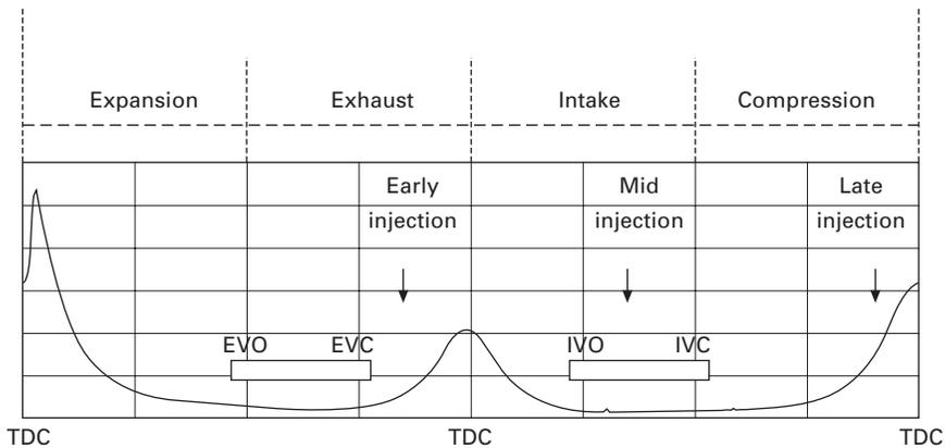
6.10 In-cylinder pressure diagram with negative valve overlap.
