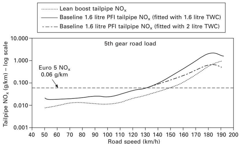
4.11 Tailpipe NO<sub>x</sub> emissions – 5th gear road load.
