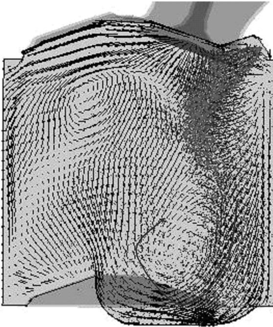
7.15 Corresponding velocity and fuel spray distribution at BDC. The intake flow pushes the fuel spray to the intake side, which causes fuel–air mixing inhomogeneity as shown in Plate II (Yi *et al.*, 2002).
