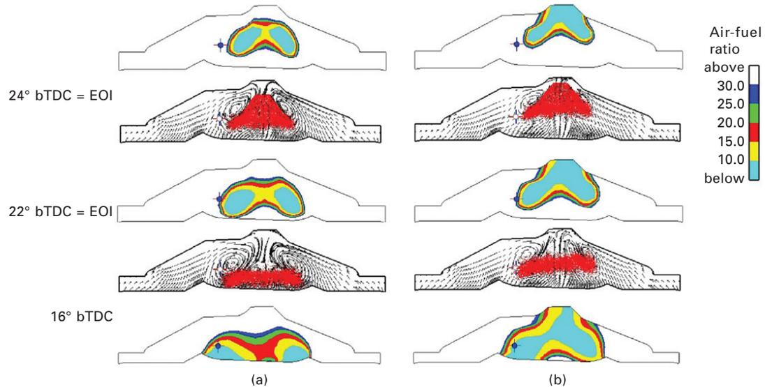
**Plate IX** Computed air-fuel ratio distribution and superimposed spray and gas velocity vector fields in the central cutting plane with (a) initial injector position, and (b) injector position raised up 4 mm along the injector axis. The cross with the blue dot in the middle corresponds to the location of the spark plug. Simulation conditions: 1500 rpm, 2.62 bar BMEP, EOI = 24° bTDC, SCV closed, MAP = 95 kPa, 80° cone piezo injector (Iyer *et al.*, 2004).
