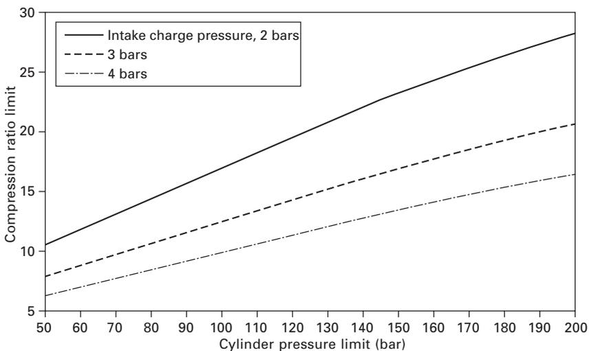
8.3 Compression ratio limit vs. cylinder pressure limit.
