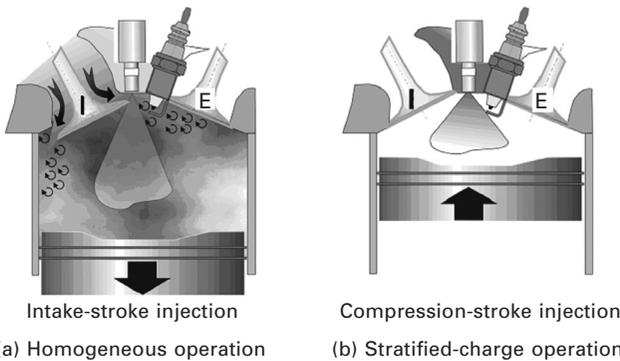
2.3 Operating modes for gasoline direct injection engines.
