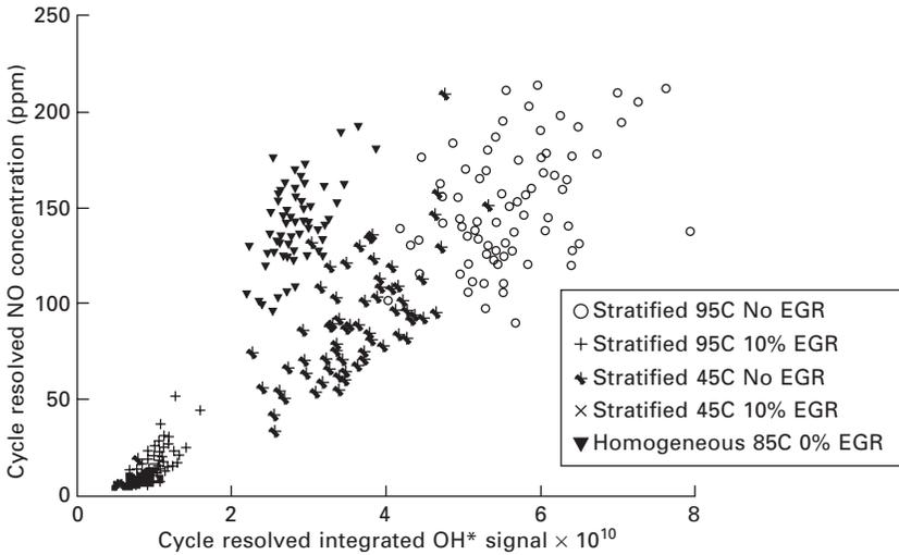
10.10 A correlation between cycle-specific engine-out nitric oxide concentration and cycle-integrated OH\* chemiluminescence for that particular cycle was observed for similar engine operating conditions. The correlation is not maintained if combustion conditions are very different (Chin *et al.*, 2008). Reprinted with permission from SAE Paper 2008-01-1072, © 2008 SAE International.
