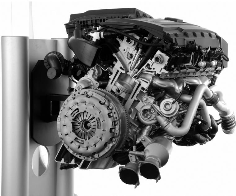
**3.16** BMW 3-litre in-line 6-cylinder twin-turbocharged engine with close-spaced piezo direct injection and twin camshaft phasing devices. This engine is arranged such that each group of three cylinders feeds one turbocharger in order to achieve pulse-division in the exhaust manifolds (courtesy BMW AG).
