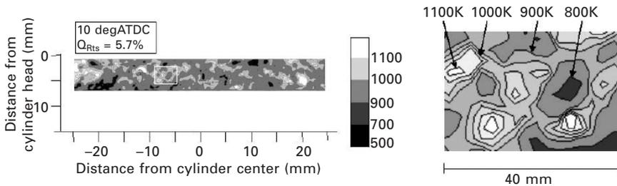
10.8 Contour images of single-shot temperature distribution at  $-10^\circ$  ATDC in HCCI combustion. The white rectangular area in the left figure is enlarged in the right figure. (Hasegawa *et al.*, 2007) Reprinted with permission from SAE Paper 2007-01-1883, © 2007 Society of Automotive Engineers of Japan, Inc. and © 2007 SAE International.
