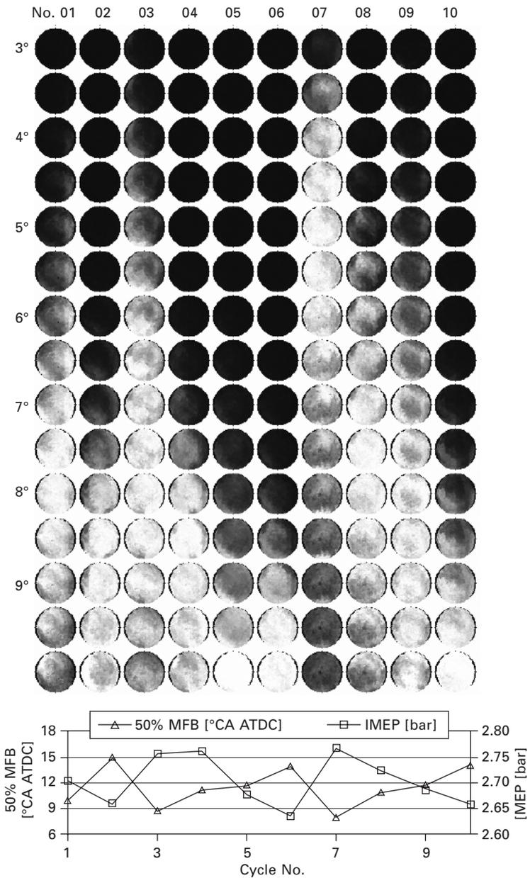
10.9 Auto-ignition and combustion progress are visualized with high spatial and temporal resolution by recording OH\* chemiluminescence with a fiber optical bundle system (Sauter *et al.*, 2006). Reproduced with permission of IOP Publishing Ltd.
