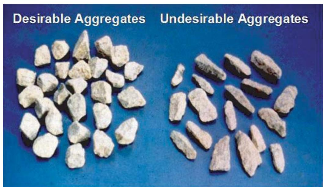
Figure 10-2. Illustration of desirable aggregate shape and angularity.
