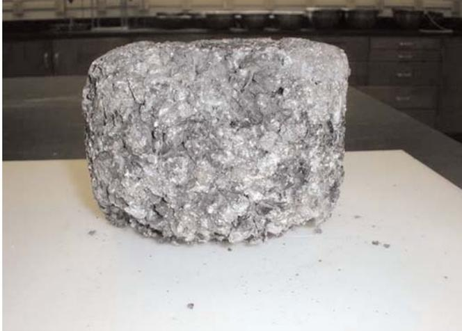
**Figure 11-5.** Illustration of sample after Cantabro Abrasion test.
