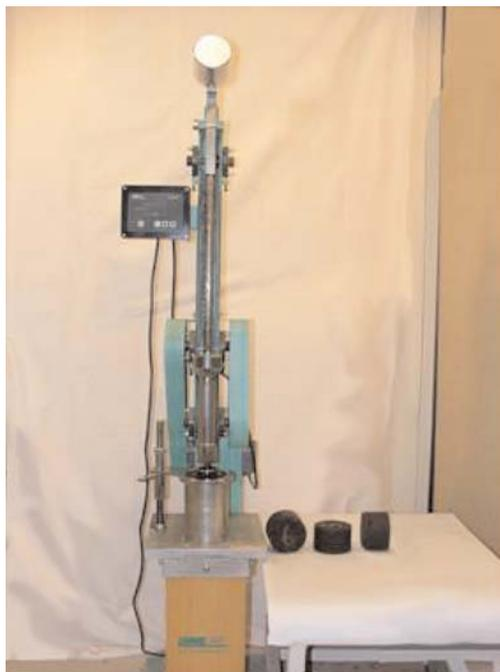
**Figure 8-1.** Marshall compaction hammer.
