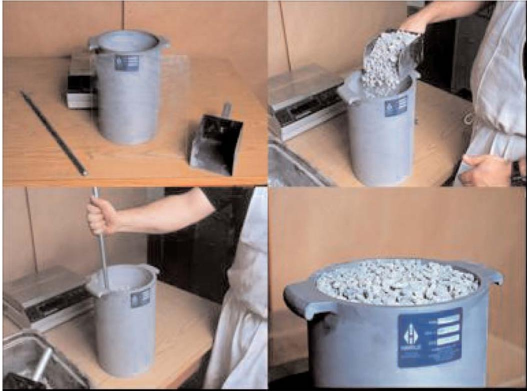
**Figure 10-5. Method of determining VCA in dry-rodded condition.**
