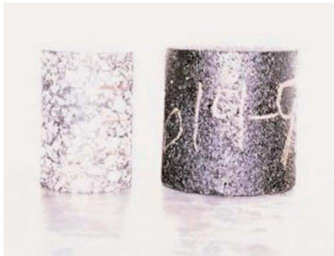
**Figure 6-3.** Photograph of an AMPT test specimen.
