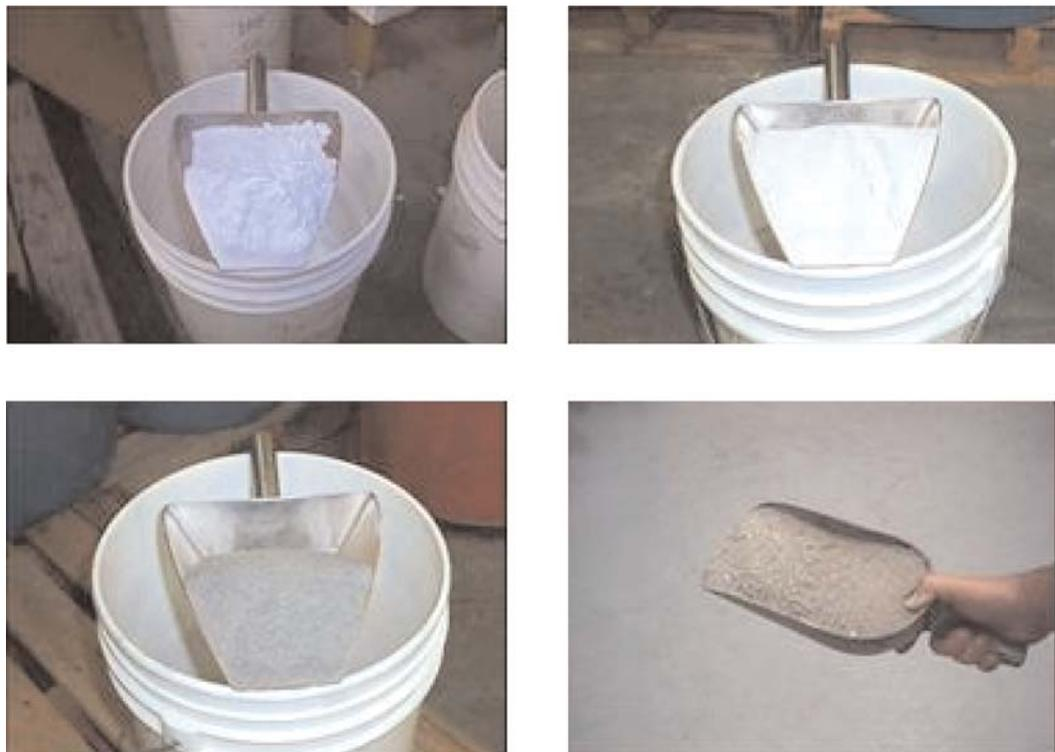
**Figure 10-3. Typical mineral fillers used in GGHMA.**
