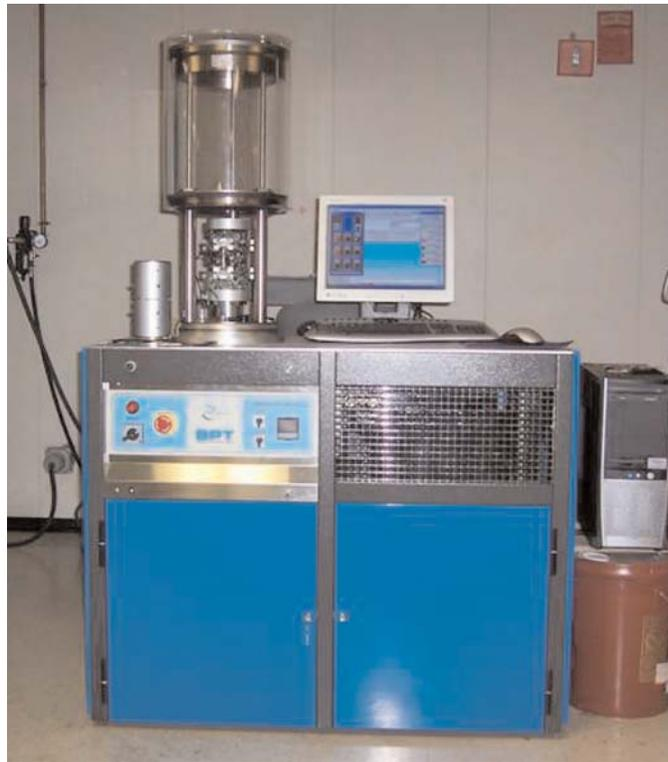
**Figure 6-1.** Photograph of a simple performance test system.
