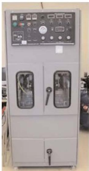
**Figure 6-5. Photograph of the asphalt pavement analyzer.**
