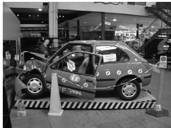
Fig. 1.6 Crumple zone — impact test at the British Transport Research Laboratory (TRL) Image Courtesy of StaraBlazkova at the Czech language Wikipedia
