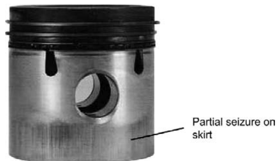
Fig. 3.23 Damage at piston skirt
