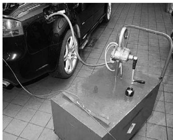
Fig. 7.7 Fuel retriever equipment (HSE). Note metal collection tank and earthing straps
