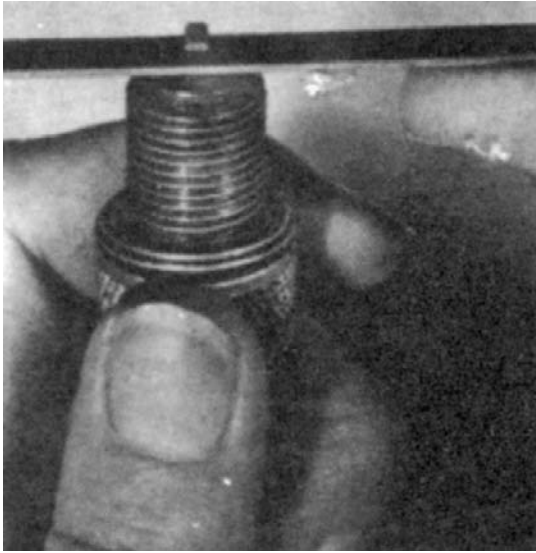
Fig. 27.53 Filing the electrodes
